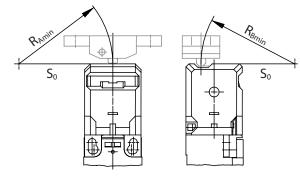
$R_{\text{Amin}}$  and  $R_{\text{Bmin}}$  depend on the actuator. Applies accordingly also to lateral retraction directions.
